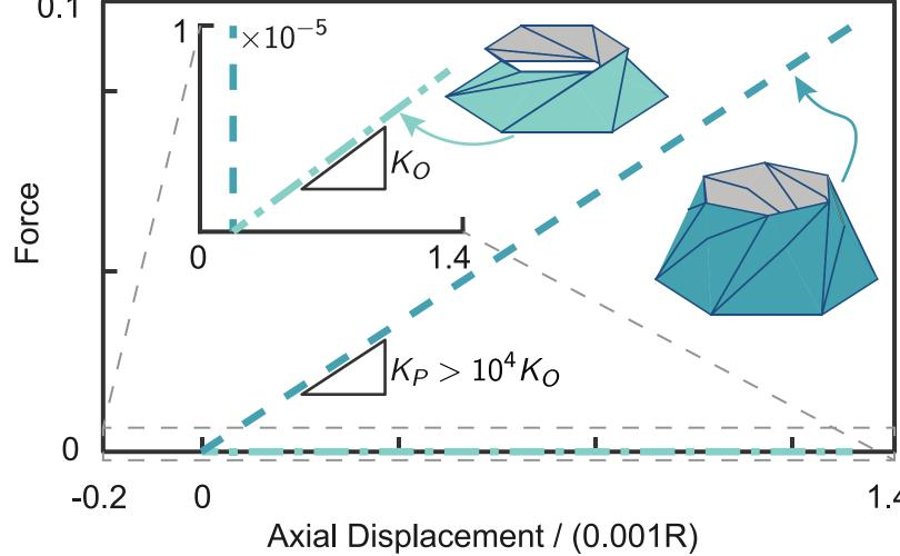
The flexible deformation mode is dominated by crease folding, while the stiff mode requires more panel stretching.
