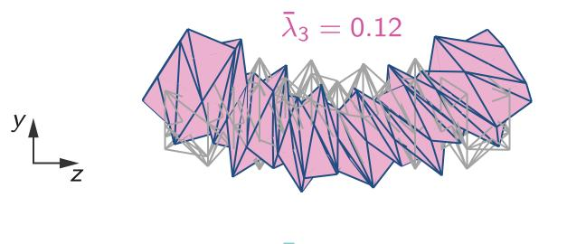
Bending stiffness (reflected by the eigenvalue) of the Kresling tube can be tuned as the constituent units switch among different stable states.
